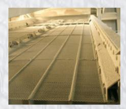
The use of anti-clogging wire screens avoids the clogging and plugging of materials in meshes.
